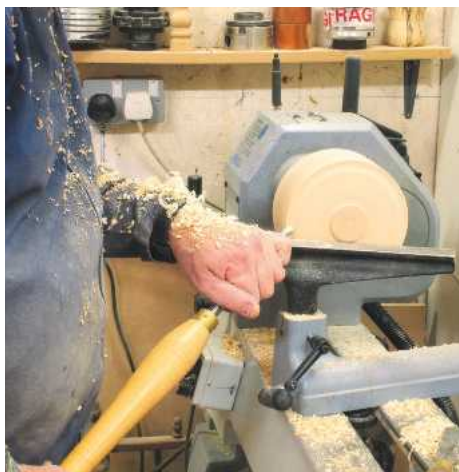
▲ Pic.4 Initial shaping of the blank using the gouge is done with the handle low down and the flute of the tool pointing at 10 o'clock. The shavings should be exiting the flute of the tool when it's in the correct position
